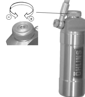
With the adjuster you optimize the suspension for your driving style and the road conditions.
