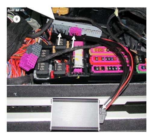
Fix the control box with hook-and-loop tape.
