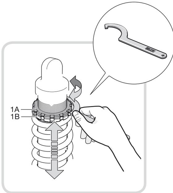
*Spring Preload, the difference between A and B:*
